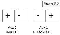
In order to select operation of Aux 1 between relay contact or 12v output JP6 and JP8 need to be configured accordingly following the instructions provided in this section. (Set for dry contact by default)
